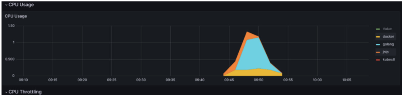
Figure 8 CPU Usage of Build Agent containers during pipeline execution
